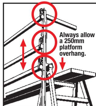
10. While you are standing on the ground, insert one end of the guardrail into the yoke provided.
