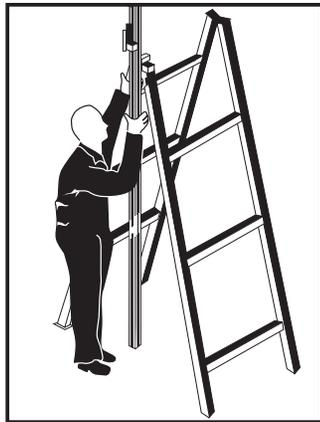
6. Fit spreader bar with trestle in fully open position. Make sure steel tongue fits up into the slot provided in "Master Post". Tighten handles.
