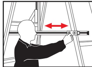
7. Slide spreader bar jaws outward until hard up against trestle legs. Tighten handles.
