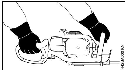
Right hand on the control handle and left hand on the front handle.
